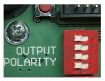
Output Polarity dip switches. (Also used to set flashing outputs in programming mode). Input connections: Inputs activating the red output -1, 2, 4, 5, 6 Input activating the yellow output -3
