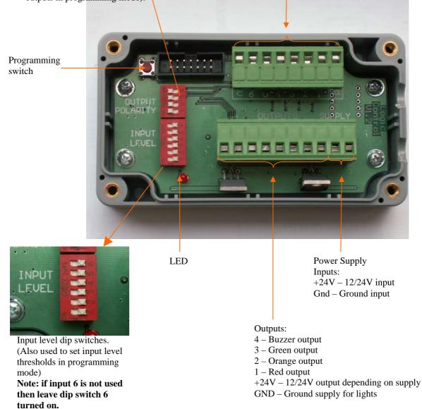
Figure 1. Layout of Universal Light Control Module
